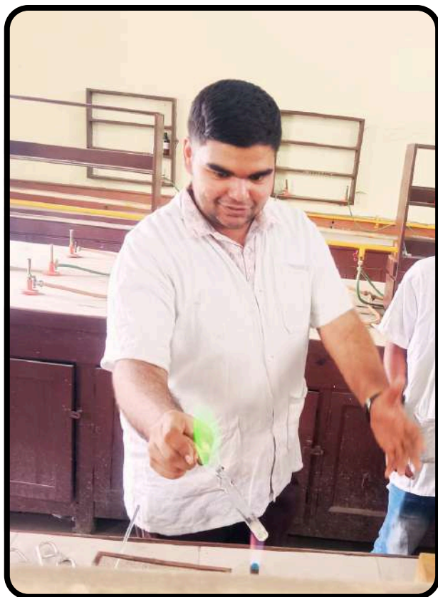
Photo 5: Green-edge flame in Borate detection test
