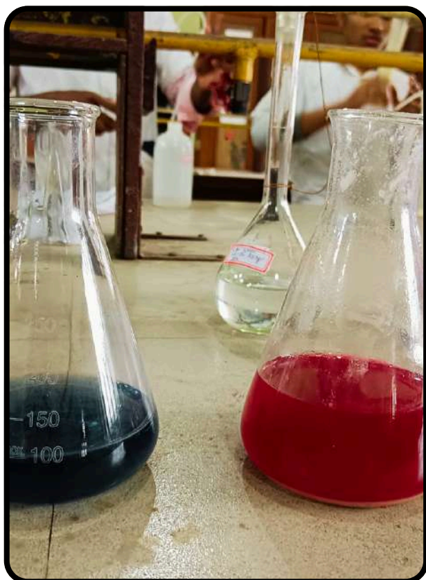
Photo 9: Colours of complexometric titration
